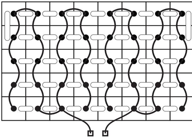
*Note: Batteries larger than 24 Cell / 48 Volt require two separate plumbing systems to be installed to ensure proper filling.*
