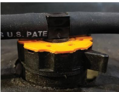
**3.** Reference the installation diagram and install the 4 pre-cut tubing assembly segments onto each row of valves. Align the swivel tees onto the top of each
