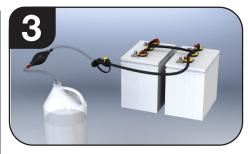
Squeeze the bulb with firm pressure to begin pumping water into the battery cells. When the bulb becomes hard, all cells are full.
