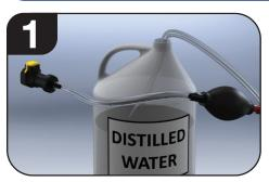
Insert the squeeze bulb filler assembly into a jug of distilled water. Prime bulb by squeezing until it is filled with water. Water jug must be left below the top of the batteries to prevent siphoning.
