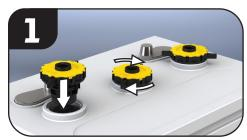
Remove existing vent covers and install Pro-Fill valves by inserting into battery and tuning 1/4 rotation to lock into place.
