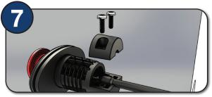
Position the nub area of the cable jacket into the plug housing body as shown and attach the housing cover with the remaining two screws (G). Assure screws are tight and there is no "slip" between the drain housing and drain cap.
