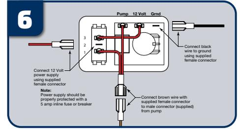
Attach wires as shown in the wiring diagram on the next page.
