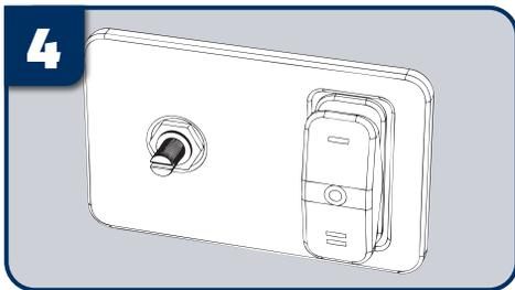
Install the timer switch from the back side and secure with the hex nuts. Snap in the master switch when using the ProTimer Plus+ as shown.
