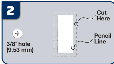
Drill a 3/8" (9.53 mm) hole for the timer. If installing the ProTimer Plus+, cut the switch hole 1/8" (3.18 mm) larger than the scribed line for clearance for the snap-in master switch mounting tabs.
