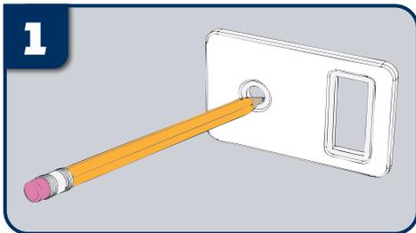
Do not remove the protective covering from the adhesive back at this time. Use the actual panel as a template to locate and mark the rotary timer switch and (for the ProTimer Plus+) the master switch mounting hole.
