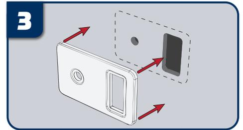
Once the holes are marked, drilled and cut, remove the adhesive backing cover sheet from the ProTimer panel and carefully align and adhere the panel in place using firm pressure.
