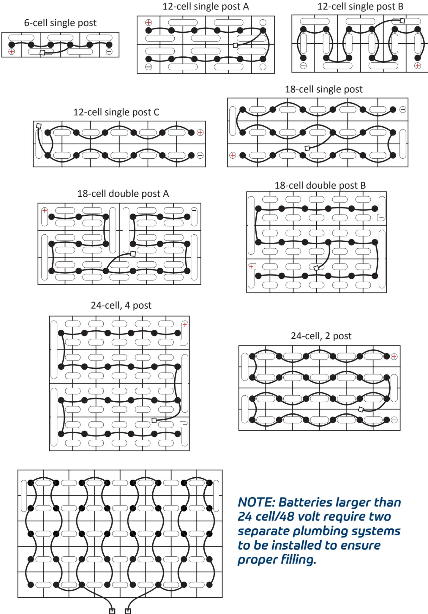
**NOTE: Batteries larger than 24 cell/48 volt require two separate plumbing systems to be installed to ensure proper filling.**
