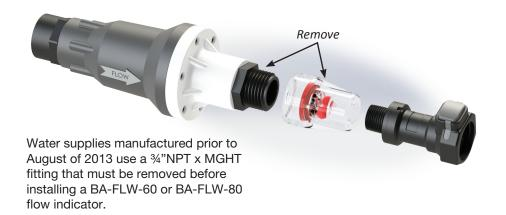
**BA-FLW-60 only:** Wrap threads 3 times with a 6" length of .5" PTFE (Teflon style) tape prior to threading into flow indicator. Tape should be wrapped in a clockwise direction and should not overlap or cover the inlet of the coupler. Coupler should be hand tightened only.
