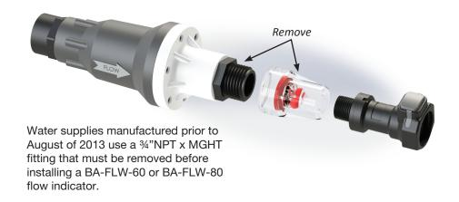
**BA-FLW-60 only:** Wrap threads 3 times with a 6" length of .5" PTFE (Teflon style) tape prior to threading into flow indicator. Tape should be wrapped in a clockwise direction and should not overlap or cover the inlet of the coupler. Coupler should be hand tightened only.
