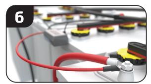
Attach the red wire to the positive terminal of the positive main battery. Connect the black wire to the negative of the negative main battery.
