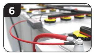
Attach the red wire to the positive terminal of the positive main battery. Connect the black wire to the negative of the negative main battery.
