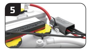
Secure the control box with a zip tie provided in a secure location.
