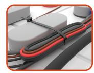
**Step 10:** Secure any loose wires with zip-ties.
