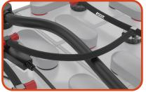
**Step 8:** Remove a red end cap from a valve near the feed tube. Install the pressure sensor with the supplied piece of tubing as shown.
