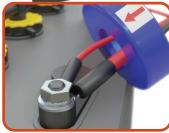
Step 2: Reinstall the nut on the red battery post and position the current sensor close to the post. Make sure your power wires are not kinked when arranging the sensor and wires.
