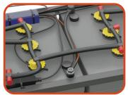
Step 5: Anchor the half voltage lead (brown wire) halfway between the positive and negative posts. Note: Coat all anchored hardware with supplied no-ox grease.
