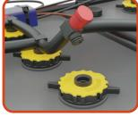
Step 6: Remove the tubing and swivel tee from a valve near the center of the battery. Make sure it is a valve in a NON-MAIN battery. (see illustration above)
