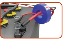
Step 1: Remove nut on the red battery post. Insert all power wires (including the Tracker red wire) through the current sensor. Make sure the red arrow on the current sensor is pointing toward the battery post.
