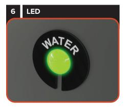
Find a location to mount the LED indicator and drill a 1/2" hole Insert the LED through the hole and place the mounting plate over the LED as shown. Remove the adhesive backing and carefully press the assembly into place.
