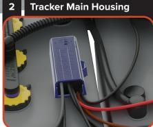
Find a secure location for the Tracker main housing. On top of the battery is preferred. If it is installed securely with zip ties, any flat surface would work.
