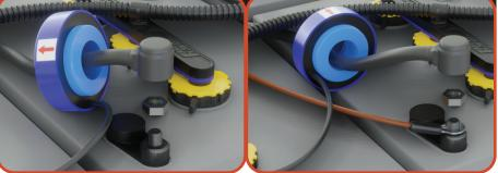
Disconnect one end of a battery connector cable in the middle of the battery pack. Insert the battery connector cable through the current sensor with the arrow indicator pointed toward the positive terminal as shown. Connect the brown wire ring to the terminal and reconnect the connector cable.
