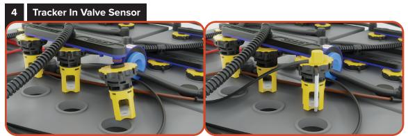
Remove a valve/manifold assembly from a center battery. Detach and discard one valve from the end of the manifold and replace with the Tracker in-valve sensor.
