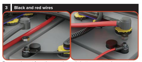
Remove the nut from the negative main battery post and connect the Tracker black wire ring. Replace the nut. Remove the nut from the positive main battery post and connect the Tracker red wire ring. Replace the nut.
