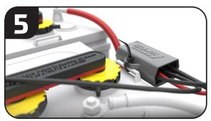
Secure the control box with a provided zip tie in a secure location.
