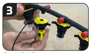
Snap the Eagle Eye sensor in the open space on the flex manifold.
