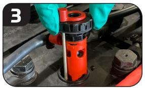
Replace with the sensor valve as shown. Use care when helping the probe find its way into the cell.
