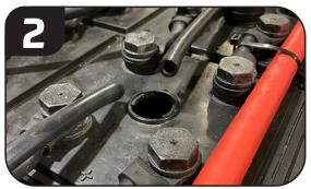
Once you have selected a centrally located valve, remove the swivel tee and valve.
