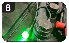
Position the LED light in a visible location and attach with a zip tie.
