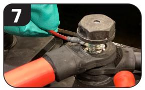
Attach the red wire to the positive post and the black wire to the negative post of the battery. Tighten firmly.
