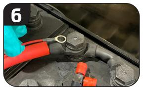
For attaching the red and black wires, remove nuts on each battery post. We recommend powering over the entire battery up to 48 volts.
