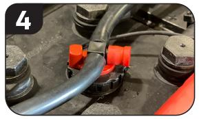
For EA-224 and EA-225, rotate clockwise to lock the valve in place and reinstall swivel tee. For EA-222 and EA-223, simply push-in the valve until it snaps in to the battery.
