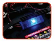
Step 3: Find a secure location for the Tracker main housing. On top of the battery is preferred. However, if it is installed securely with zip ties, any flat surface would work.
