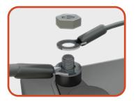
**Step 4:** Remove the nut on the black (-) battery post. Install the Tracker black wire ring terminal on the post and reinstall the nut.
