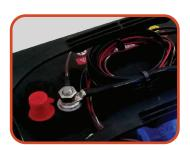
**Step 6:** Secure any loose wires with zip-ties.
