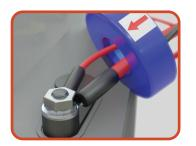
**Step 2:** Reinstall the nut on the red (+) battery post and position the current sensor close to the post. Make sure your power wires are not kinked when arranging the sensor and wires.
