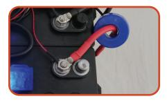
**Step 1:** Remove nut on the red (+) battery post. Insert all power wires (including the Tracker red wire) through the current sensor. Make sure the red arrow on the current sensor is pointing toward the battery post.
