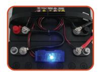
**Step 5:** Anchor the half voltage lead (brown wire) halfway between the positive and negative posts. *Note: Coat all anchored hardware with supplied dielectric grease.*
