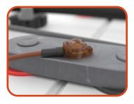
**Step 5:** Anchor the half voltage lead (brown wire) to an inter-cell connector halfway between the positive and negative posts. Coat all anchored hardware with supplied no-ox grease.
