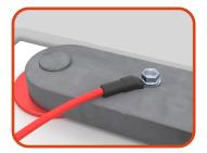
**Step 4:** Using the supplied self tapping screws, anchor the positive lead (red wire) to the positive battery post and the negative lead (black wire) to the negative post.
