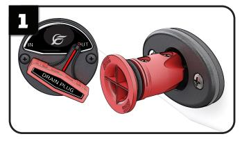
**Step 1** Move the remote drain plug actuator to the "out" position. The plug should have sufficient extension to be able to remove the plug screws and plug. If additional length is needed, it may require removing the black drain housing cap for further cable extension (inside the bilge area, see Step 4 image).
