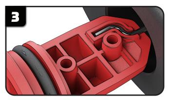
**Step 3** Take the new plug assembly and carefully lay the "Z" bend of the control cable into the "Z" groove molded in the replacement plug body as shown. Install and secure the plug cap with the (2) screws supplied (do not over tighten) (see Step 2 image). Assure that screws are tight and there is no "slip" between the plug and the plug cap.
