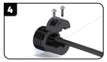
**Step 4** If the drain housing cap was removed, reposition the enlarged nub area of the control cable jacket into the drain housing body as shown. Re-install the drain housing cap with the (2) screws that were removed (do not over tighten). Assure the screws are tight and there is no "slip" between the drain housing and drain housing cap.
