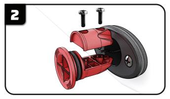
**Step 2** Disassemble the red plug assembly by removing the (2) plug cap screws installed, pull off the cap, and remove the plug. Discard the old plug.
