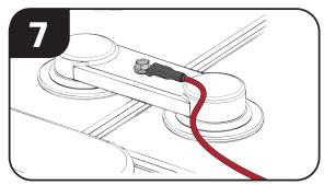
Tighten the screw. Note: Ring terminal should face down with the wire exiting at the middle of the intercell connector as shown. Apply grease to connection after securing to battery and reinstall shroud without pinching wire.
