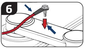
Remove the terminal shroud and screw the positive wire lead directly into the positive terminal with the included self-tapping screw.
