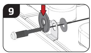
Insert bracket between the cell and battery tray on the outside edge of the battery. Insert light through the hole in the bracket and place the slotted washer over the wire as shown.
