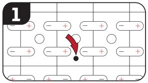
Choose probe location near the center of the battery. Drill ½" diameter hole in the cell cover with approved drill bit. Make sure there is clearance down to the plates and around the probe before drilling.
