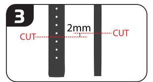
Count the same number of holes on the gauge guard starting from the bottom and cut the gauge guard at this height. Cut the sensor probe 2mm shorter than the gauge guard, then strip the heat shrink of the probe by approximately 5mm.
