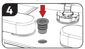
Install grommet into cell.
