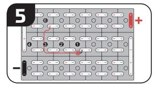
Select cell post locations for wire installation. This will require 6 cells in series with the black wire attached to the negative terminal into which the sensor is installed and the red wire attached to the positive terminal six cells up. NOTE: The wires should not be pulled tight.
