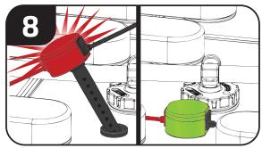
The light should now be blinking red. Insert the probe into the grommet. If the electrolyte level is normal, the light will turn to steady green.
