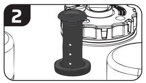
Place the gauge guard into the drilled hole until it stops. Count the number of visible holes on the gauge guard. If the guard does not have any visible holes, remove the guard and proceed to step 4.
