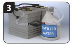
Squeeze the bulb with firm pressure to begin pumping water into the battery cells. When the bulb becomes hard, all cells are full.
