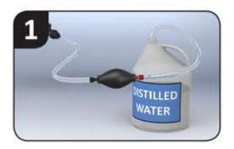
Insert the squeeze bulb filler assembly into a jug of distilled water. Prime bulb by squeezing until it is filled with water. Water jug must be left below the top of the batteries to prevent siphoning.
