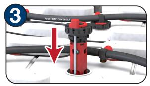
Replace with the sensor valve as shown. Use care when helping the probe find its way into the cell.
